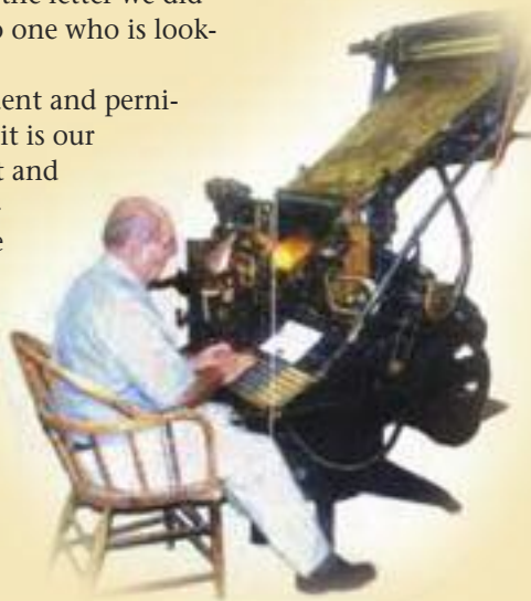
A Mergenthaler Linotype machine was industry standard for setting type until the advent of phototypesetting in the 1970s.
